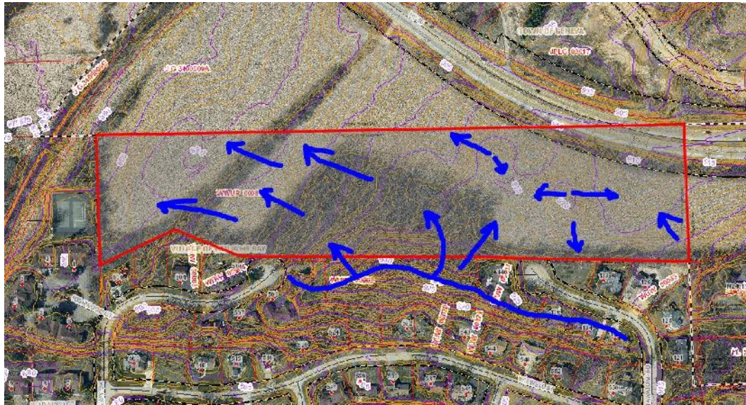
Existing Drainage Pattern
