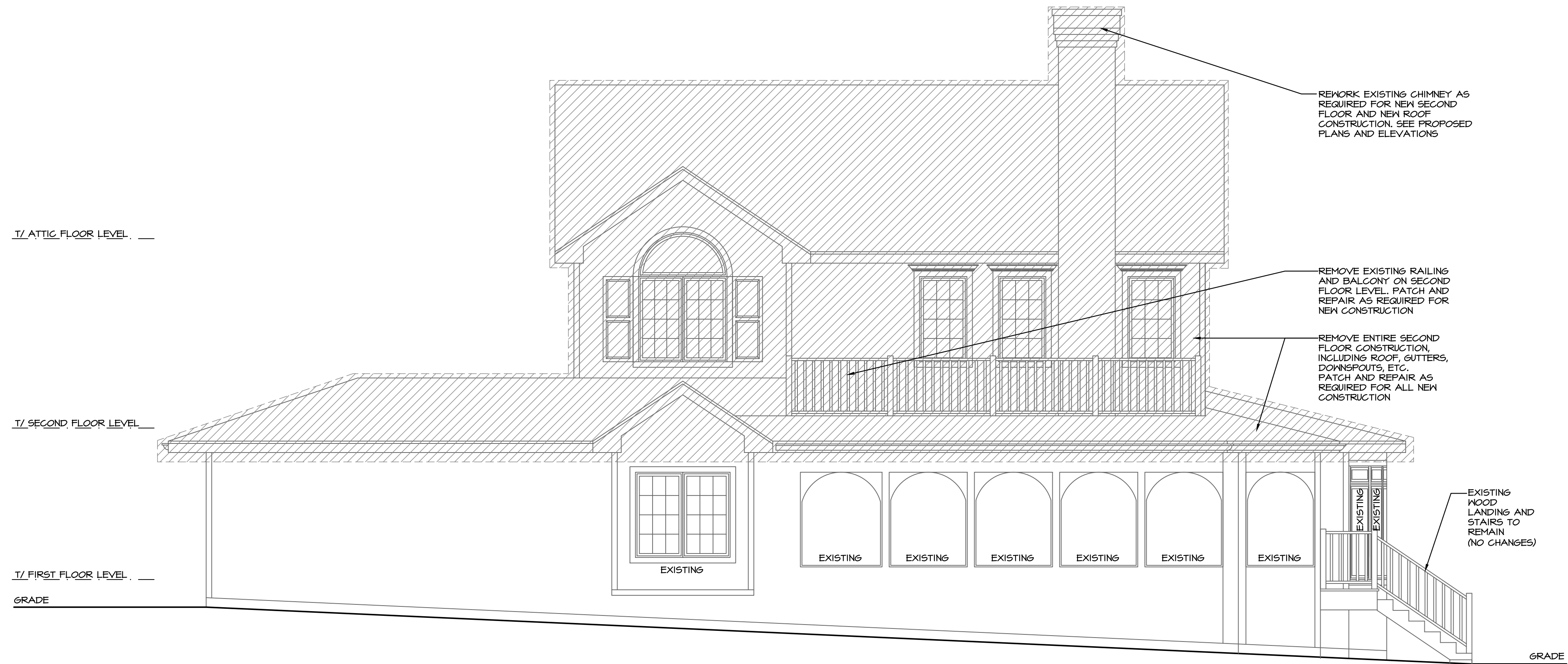
2 EXISTING LEFT ELEVATION A 03 DEMOLITION
