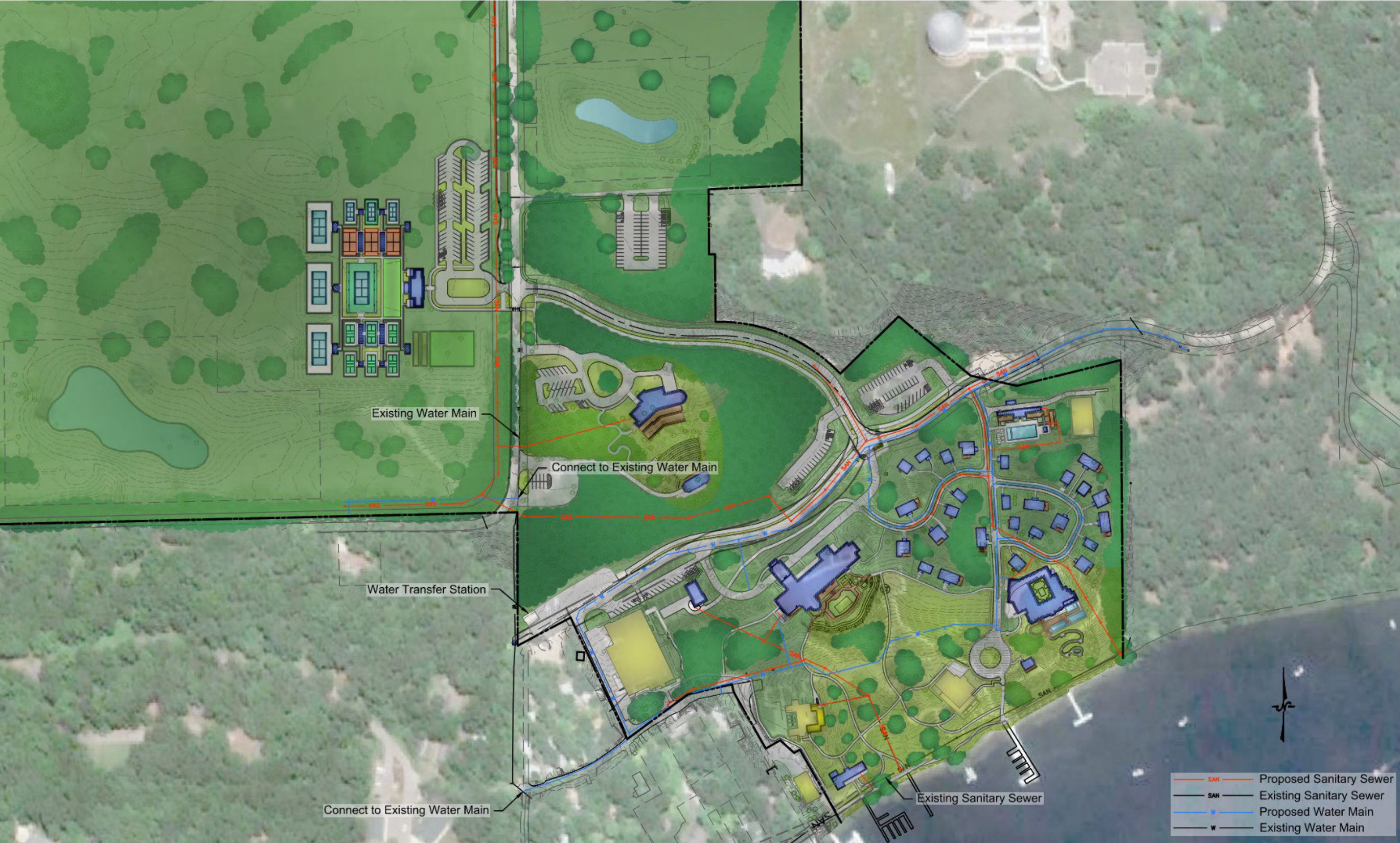
PROPOSED UTILITIES DIAGRAM SCALE: 1" = 225'
