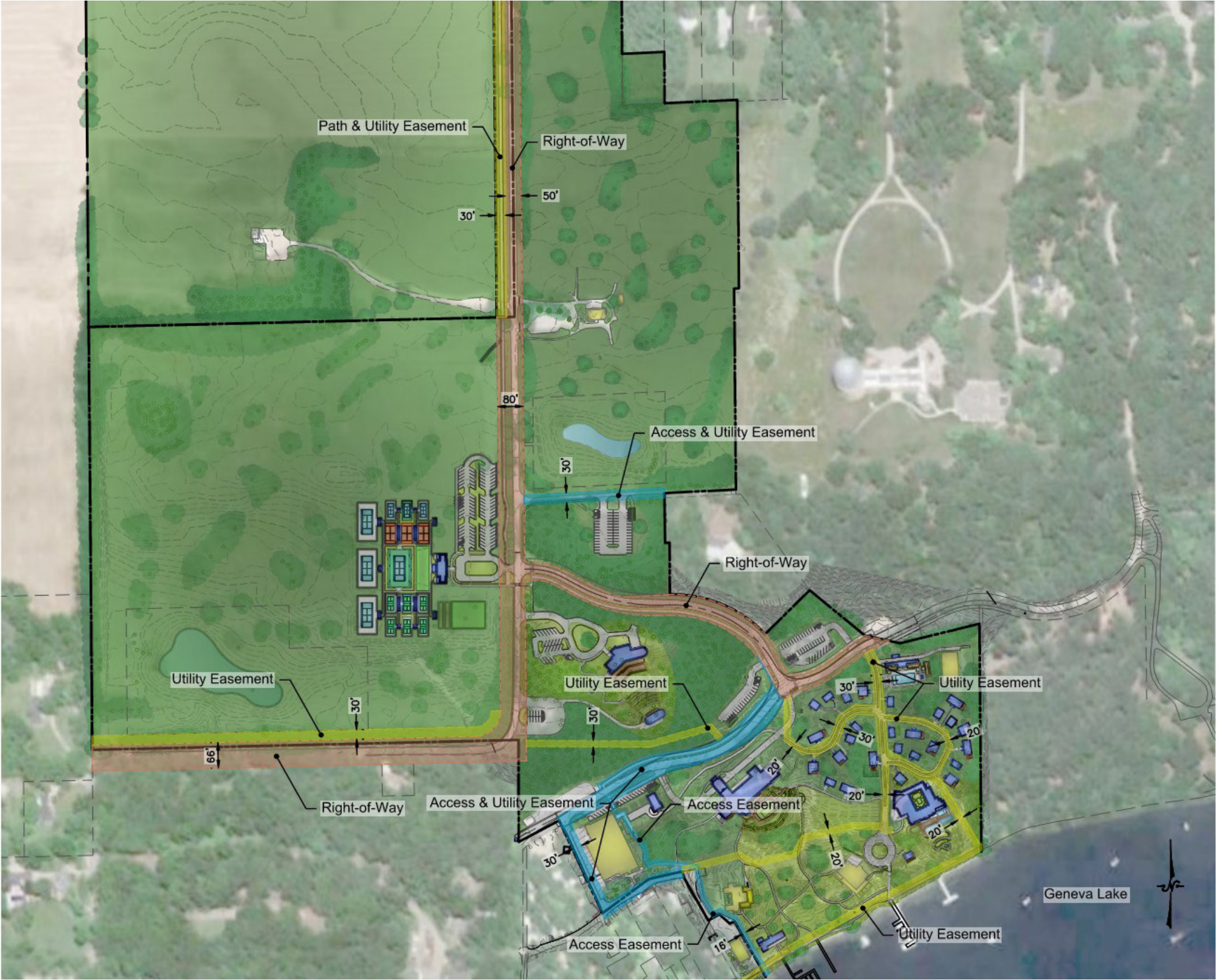
PROPOSED RIGHT OF WAYS AND EASEMENTS DIAGRAM SCALE: 1" = 350'
