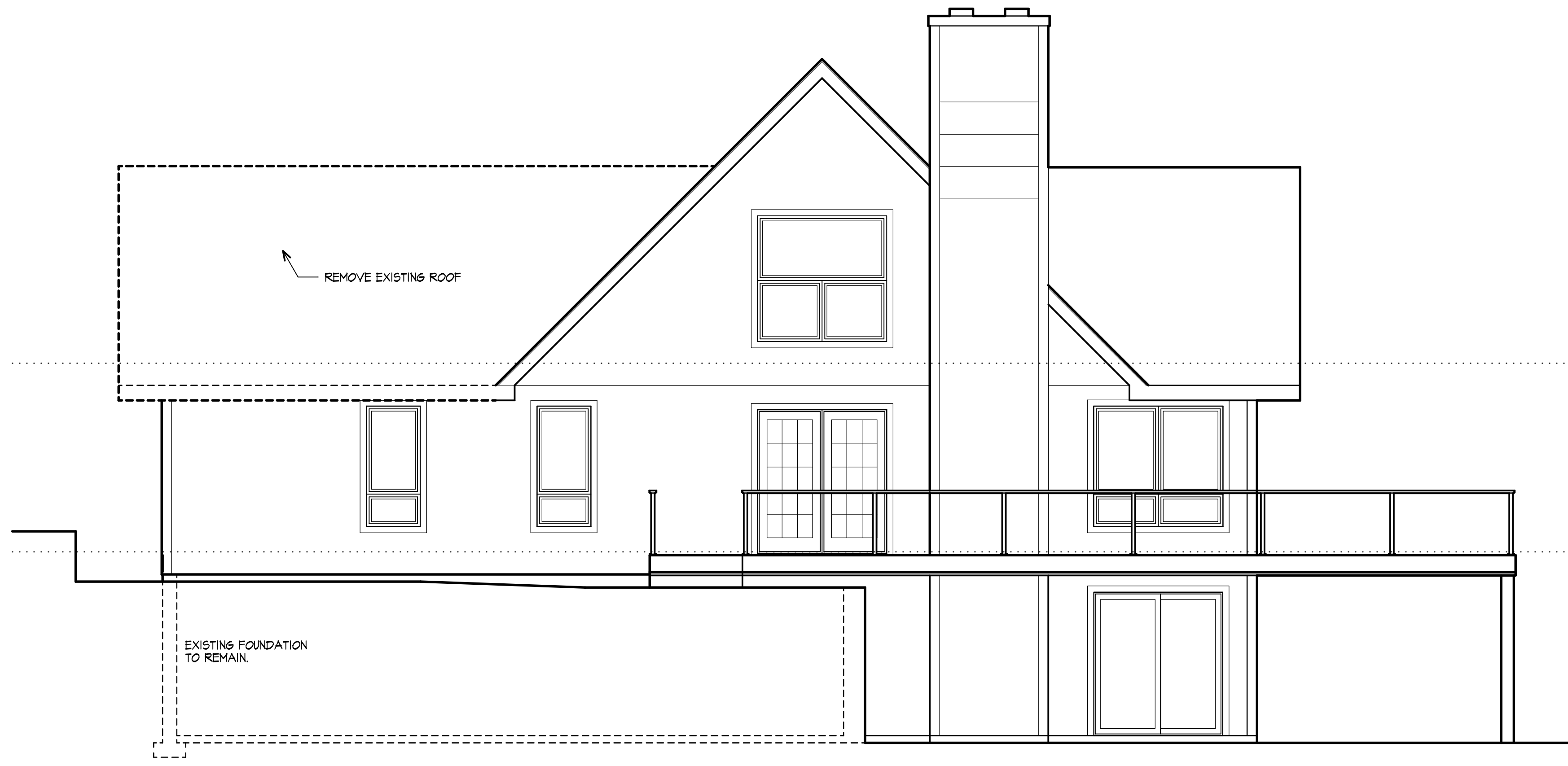
Existing Front Elevation 1/4"=1'-0" 0 1 2 4 6 8
