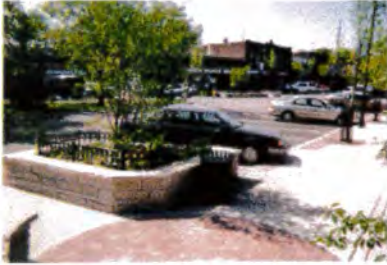
CURB BUMP-OUTS ARE DEFINED WITH LIMESTONE WALLS, DECORATIVE PAVING, AND ORNAMENTAL PLANTINGS
