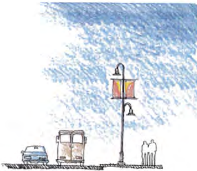
OVERHEAD ROADWAY LIGHT POLE WITH 5' HT. RECTANGULAR BANNERS AND MATCHING DECORATIVE PEDESTRIAN LIGHT FIXTURE
