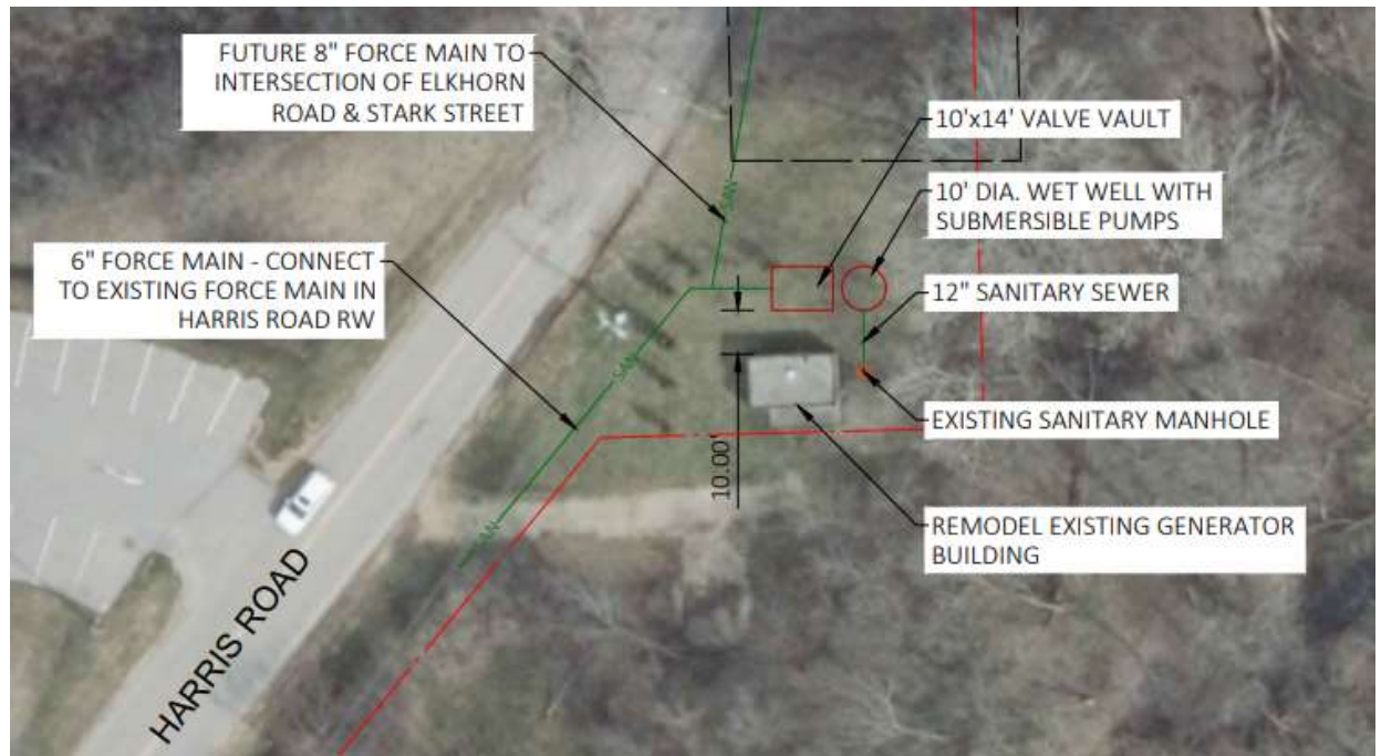
Figure 7 – Lift Station Upgrade Concept
